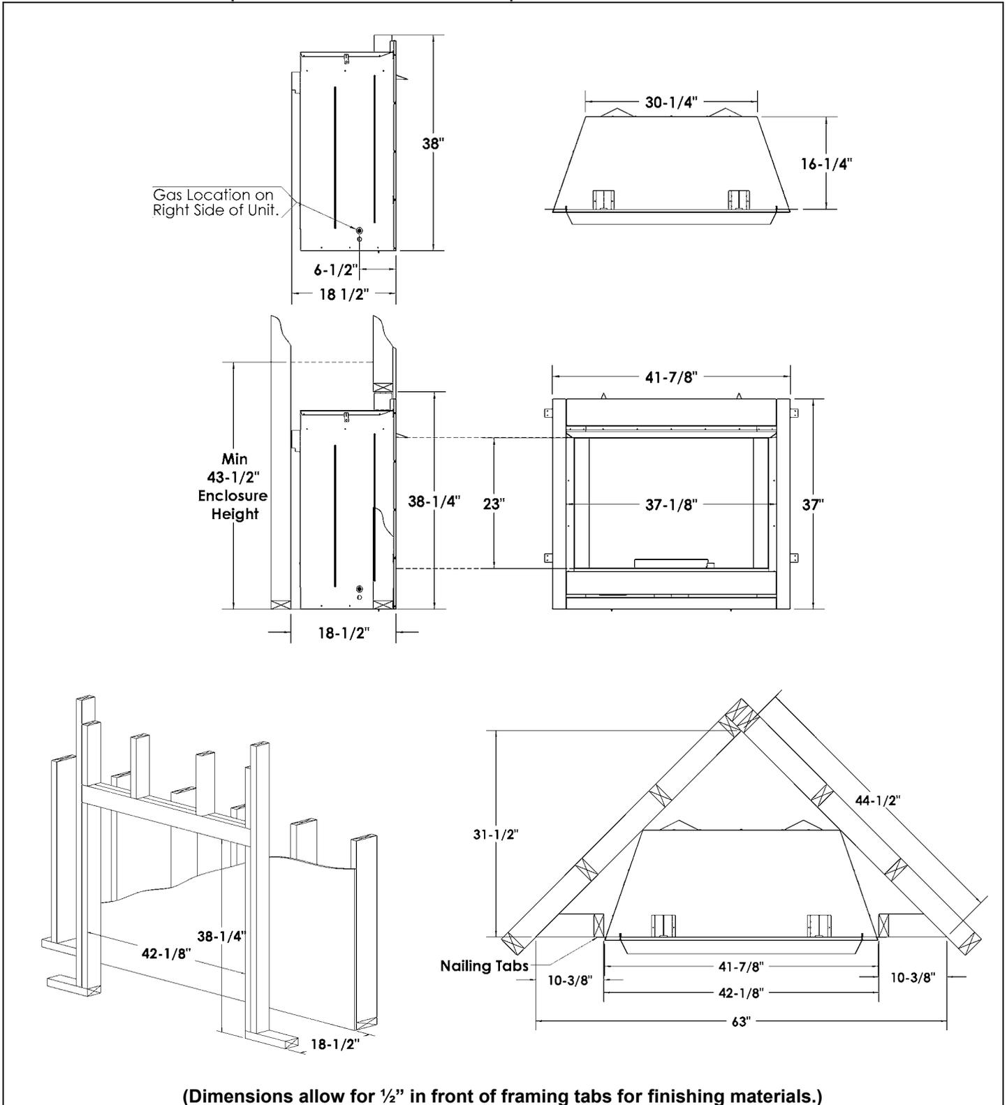
(Dimensions allow for 1/2" in front of framing tabs for finishing materials.)
