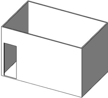
Walls on all sides (Minimum area of 96 square feet), but with no overhead cover and at least one permanent opening (doorway) at ground level.
