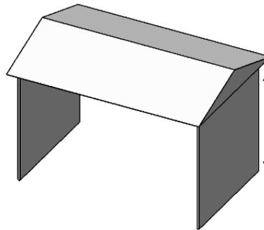
Minimum Side Wall Height is 78" from bottom of unit.
