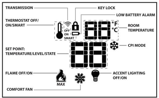
Figure 2: Proflame 2 LCD screen details.
