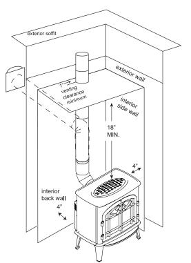
Figure 21: Trenton clearance to combustibles.
