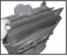
Figure 38: Trenton safety screen removal.
