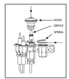
Figure 74: Pilot hood and orifice.
