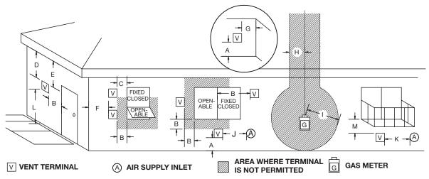
Figure 24: Minimum clearances to vents.
