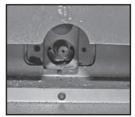
Figure 75: Orifice from inside the firebox.
