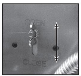
Figure 69: Venturi adjustment.
