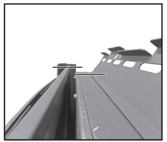
Figure 57: Improper seating of safety screen.
