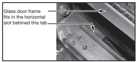
Figure 53: Glass door positioning.
