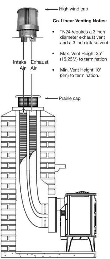
Figure 26: Trenton co-linear venting configuration.
