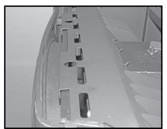
Figure 61: Screen holder in correct position.
