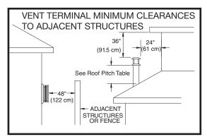
Figure 23: Clearances to adjacent structures.
