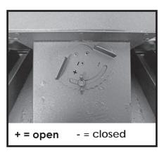
Figure 68: Trenton damper adjustment.
