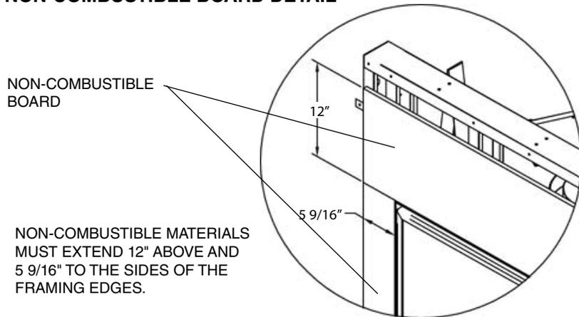
NON-COMBUSTIBLE MATERIALS MUST EXTEND 12" ABOVE AND 5 9/16" TO THE SIDES OF THE FRAMING EDGES.
