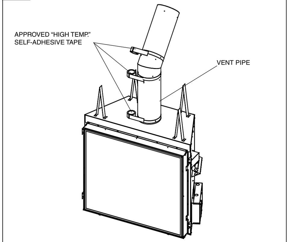
All outer joints of the vent pipe must be sealed with the approved "High Temperature" self-adhesive aluminium tape provided. Wrap the tape completely around the joint and press firmly in place.
