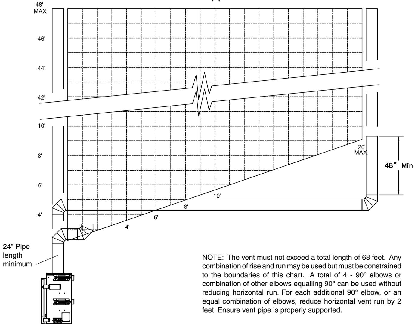
NOTE: The vent must not exceed a total length of 68 feet. Any combination of rise and run may be used but must be constrained to the boundaries of this chart. A total of 4 - 90° elbows or combination of other elbows equalling 90° can be used without reducing horizontal run. For each additional 90° elbow, or an equal combination of elbows, reduce horizontal vent run by 2 feet. Ensure vent pipe is properly supported.
