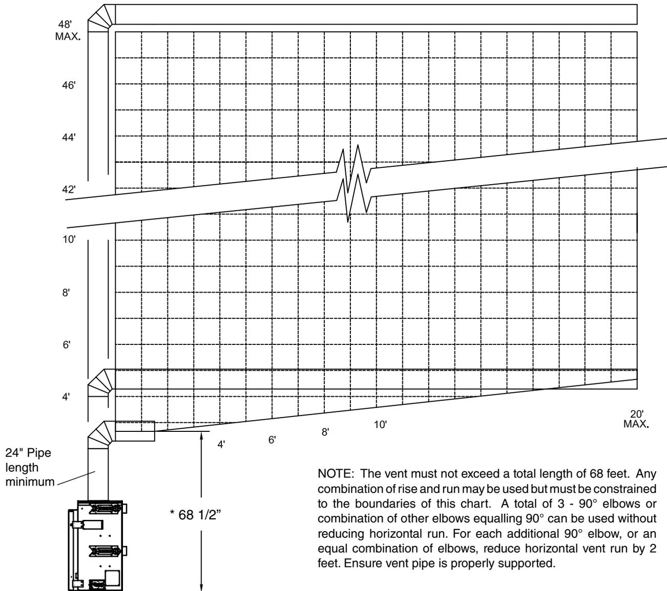
**NOTE:** The vent must not exceed a total length of 68 feet. Any combination of rise and run may be used but must be constrained to the boundaries of this chart. A total of 3 - 90° elbows or combination of other elbows equalling 90° can be used without reducing horizontal run. For each additional 90° elbow, or an equal combination of elbows, reduce horizontal vent run by 2 feet. Ensure vent pipe is properly supported.
