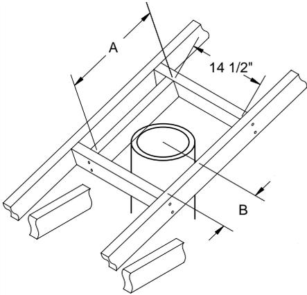
**Size of the opening will have to increase with the pitch of the roof to ensure a 1 3/4" inch air space clearance between vent pipe and combustibles.**
